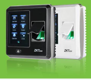
The SF300 is an IP based fingerprint terminal, which operate in both network mode and standalone mode. it can connect with ZKAccess3.5 software for access control and time attendance management.
